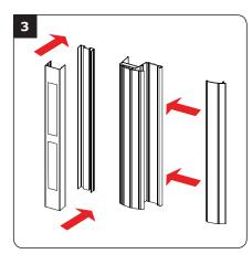
To finalise the assembly, tighten all fixings, and protect the handle fixing section by fitting the cover and end caps.
