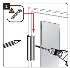
With the door closed, position the architectural handle onto the edge of the opening leaf of the door, ensuring the handle covers the box-section. Mark the vertical and horizontal holes, drill as required, then temporarily fix the handle leaving a small gap around the box section – check the alignment of the magnets in the box section with the magnets in the handle.
